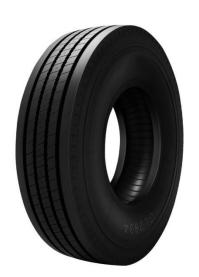
Good news, the Advance radial truck 225/70R19.5 GL283A speed rating has been increased from 75mph to 87mph!
